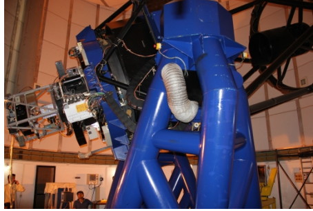
FIGURE 9.1: Observational setup of TIRCAM2 at the 2 m IGO telescope
